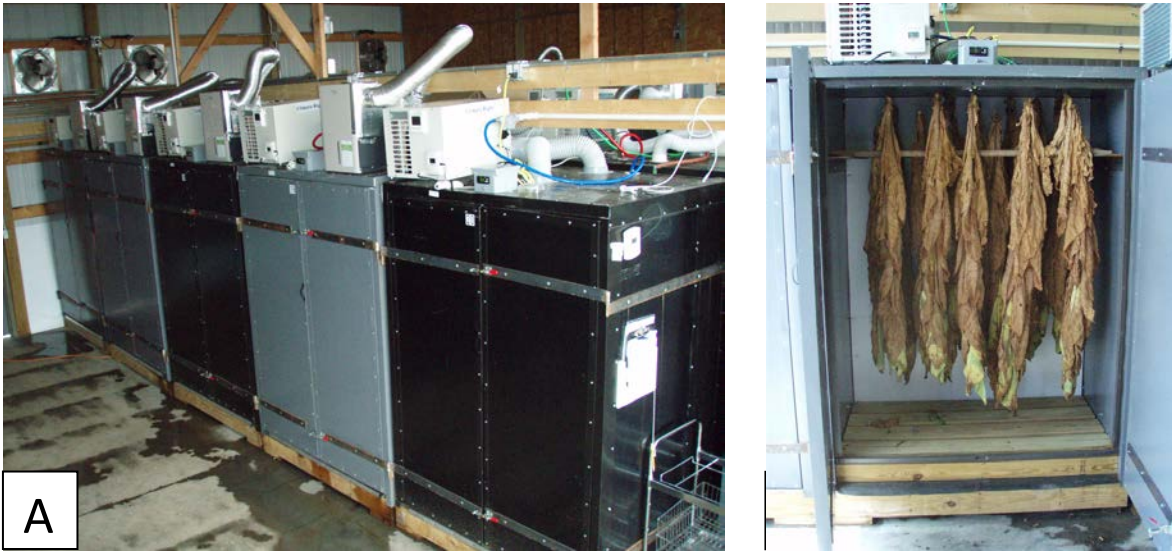
Fig. 1. A. Five of the twenty four curing chambers in purpose-built housing. The temperature and humidity in each curing chamber are controlled independently of each other. B. The airflow is directed down behind the plenum (white behind tobacco) and up through the slatted floor.
