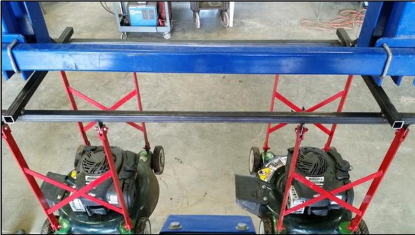
**Figure 1:** Mowers mounted on high clearance sprayer
